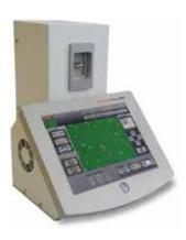
Cellometer Auto 2000 Cell Viability Counter (Dualfluorescence cell counter to analyze primary cells from peripheral blood, cord blood, bone marrow, and other complex samples)
